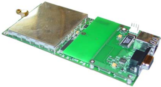
Tiamis-800 transceiver with Option 1108 - interface board
