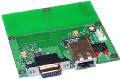
Option 1108- Ethernet /Serial Server and diagnostics port interface board
