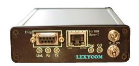
Tiamis-800 software defined radio transceiver in the enclosure when equipped with Option 12E0
