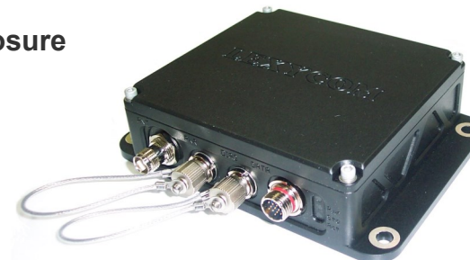
MIL-Grade, Ruggedized Enclosure 4.55" x 6.2" x 1.6" (with mounting plate), equipped with 3 circular 801 series MIL-spec connectors, 1 TNC connector
