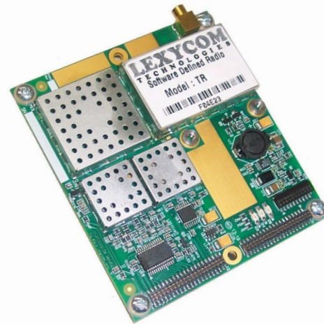
270-400 MHz Board Level Transceiver measurements: 3.18" x 2.89" x 0.47"
